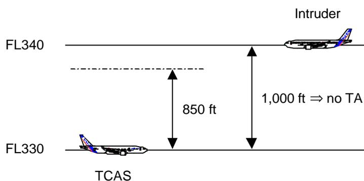
**Figure 6: standard RVSM vertical separation**
