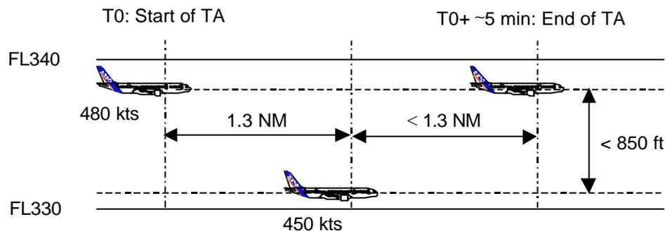
**Figure 11: low closure rate and vertical offsets**
